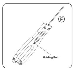
2. Attach the frame to the front fork by Inserting the Frame into the front fork.
